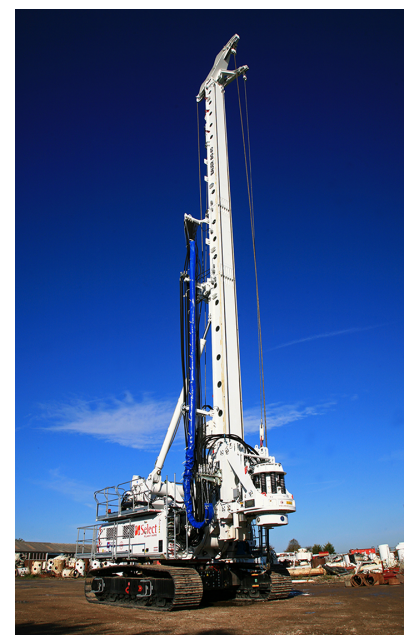
CFA Piling Rig
